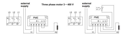
The brakes are supplied externally.
